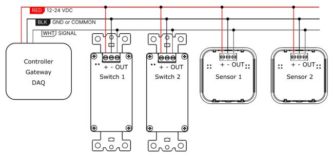
4 Wall Switch Wiring Diagram
