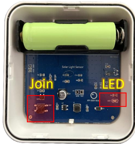
2 Join Button and LED Indicator
